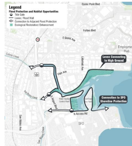
F4: Individual Tide Gates with Levee System
